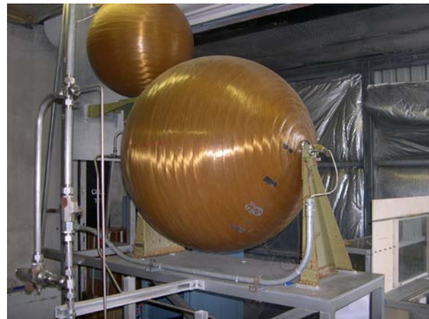
Figure 13: Orbiter MPS GHe System COPVs
